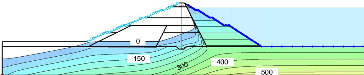
Figure 5. Piezometric line at the end of first filling
