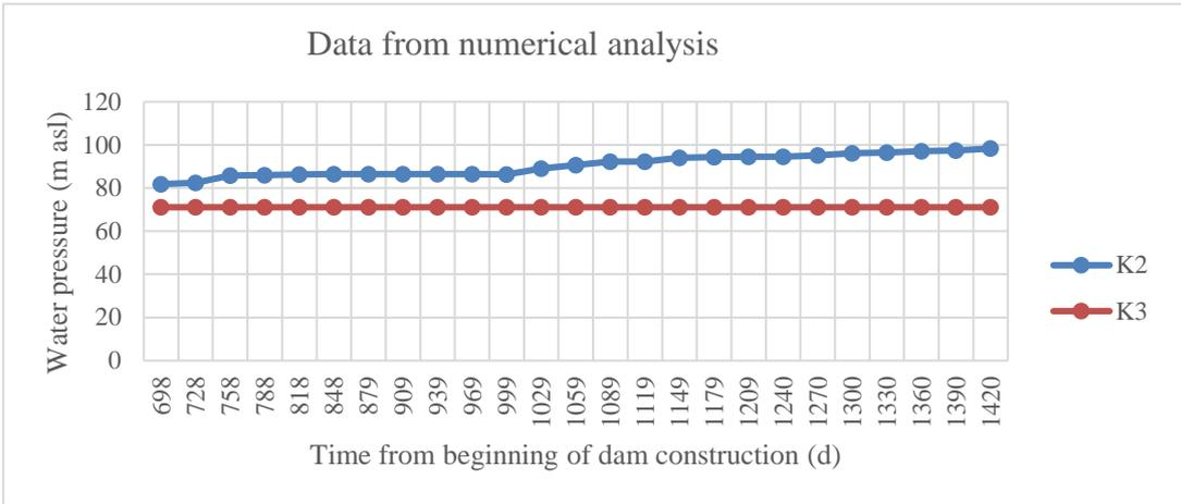
Figure 3. Water level at piezometers K2 and K3 - results obtained by numerical analysis
