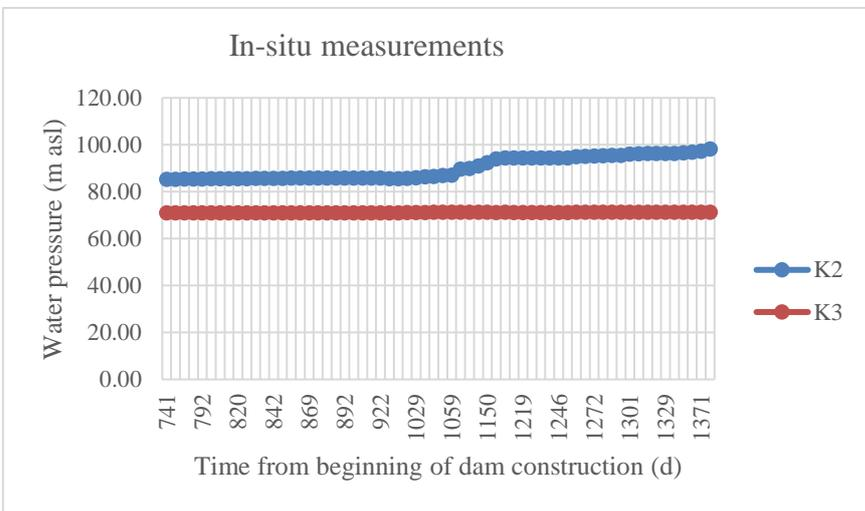
Figure 4. Water level at piezometers K2 and K3 - values obtained by in-situ measurements
