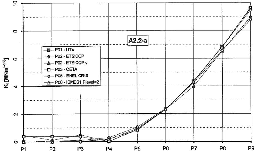
Figure 10 -  $K_I$  variation along the crack tip.
