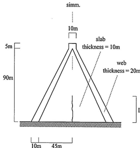
Figure 6 - Geometrical data of the ideal case proposed in the BW3.
