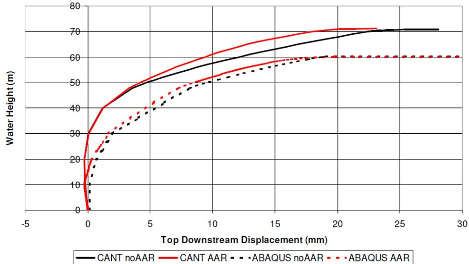
Figure 12 - Comparison of displacements at the dam crest computed with CANT-SD and ABAQUS.
