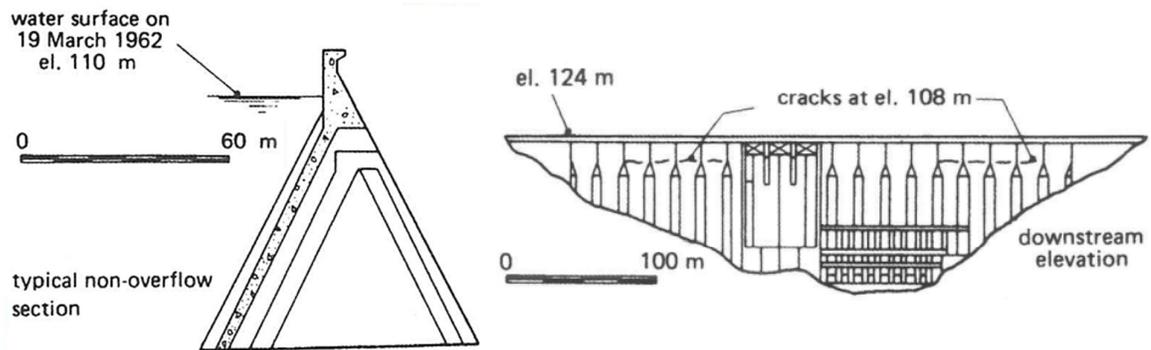
Figure 16– The Hsinfengkiang Dam after the earthquake.
