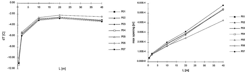
Figure 7 - Rigid foundation. Relationship between crack length and the associated critical temperature (left). Maximum openings relative to different crack length (right).
