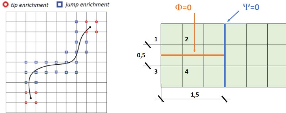
Figure 13 - An arbitrary crack on a uniform mesh (left) and the two-levels set functions generally used in XFEM to describe a crack and tracking its motion (right).
