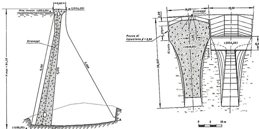
Figure 2 – Buttress dam.
