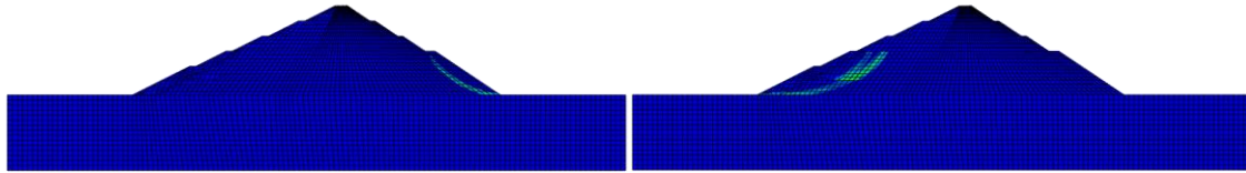
Figure 6. Contour of the plastic deviatoric strain showing the sliding surfaces at upstream (on the left) and downstream (on the right) slope.
